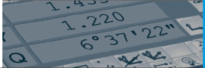
The new data processor colour touch screen, **designed and manufactured by LTF**, allows to convert the traditional profile projector in a true two-dimensional measuring instrument allowing direct measurement of the part under testing in the X-Y coordinates and angular, as well as to make program of the measuring sequence. USB, serial and LAN outputs are available to connect the M-Touch to PC and other peripherals
